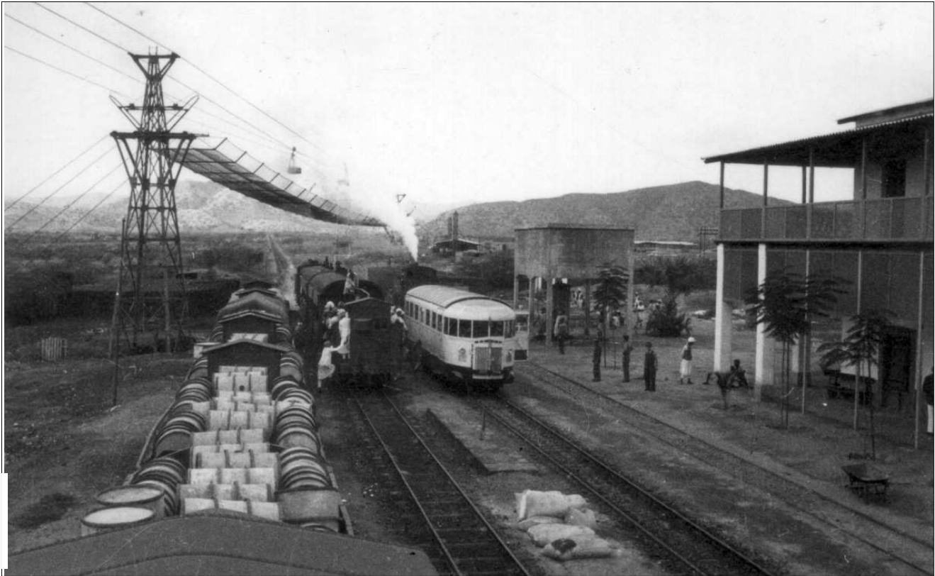
Photo taken by Prof. Gallo, Chief Engineer, sometime in the late 1930s/early 1940s. This picture depicts a train at Mai Atal. JBT comments "It shows the morning 'rush hour'. Freight trains tended to leave Massawa in the cool early morning, often double-headed. One lengthy train proceeded across the flatlands to Mai Atal. There it was split into two or three or more lots, which left later for Asmara over the steeper gradients, sometimes with a further shedding of load at Ghinda. In this photo the loads have been detached, and the loco can be seen behind the littorina, taking water and already blowing off steam before following the daily passenger train, which has already started en route to Asmara. The littorina has duly arrived from Asmara. The Ropeway appears to be in operation as a skip can be seen moving and the protective netting is in good order.
