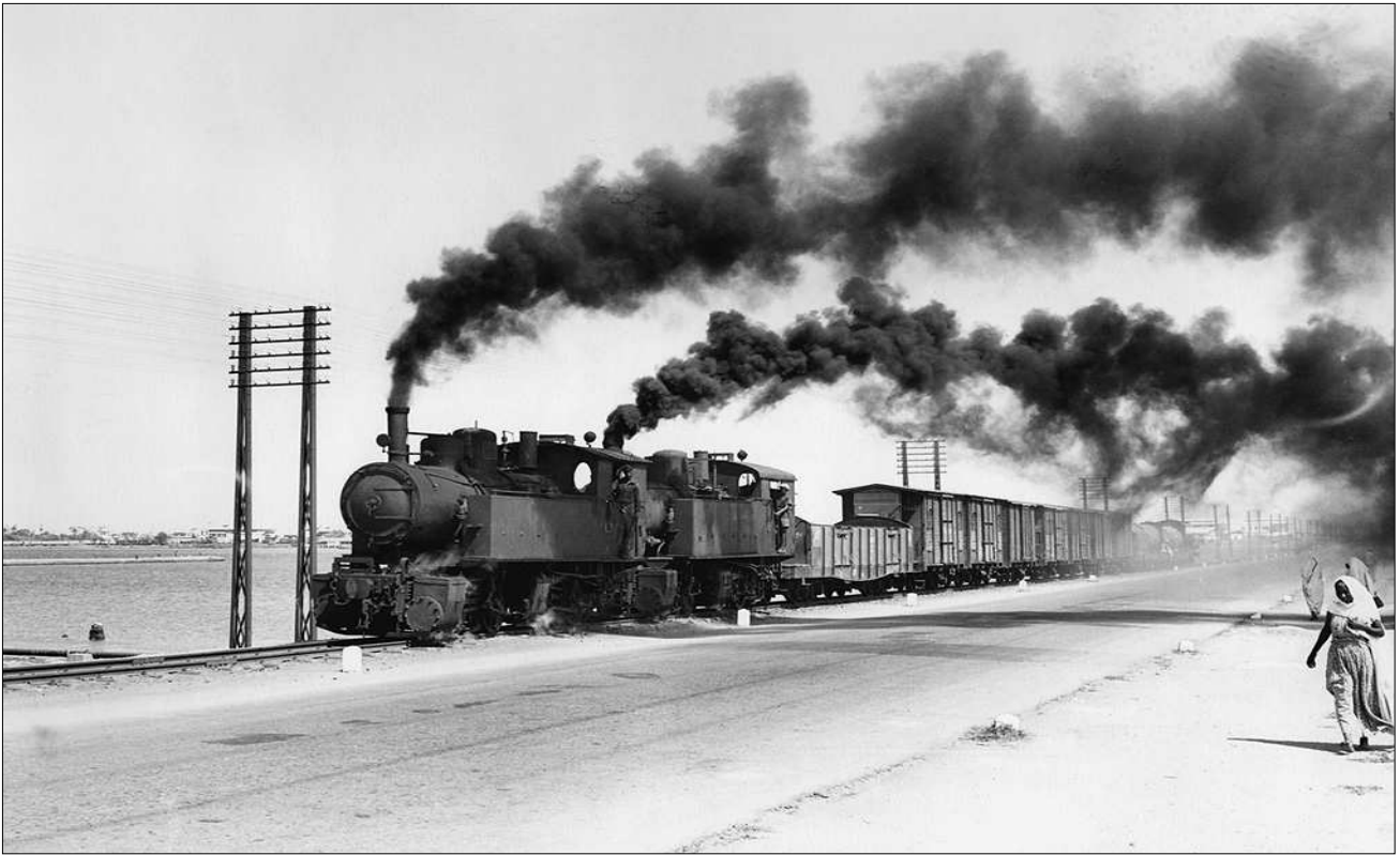
440.001 (works no 1113) and 440.004 (works no 1116), both built by Ansaldo 1914, crossing the causeway in Massawa at the start of the journey to Asmara. The length of this train illustrates the importance of the railway in carrying freight during the Ethiopian period. February 1955
